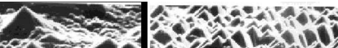
Fig.2.20. SEM picture of n type<100> Si membrane, etched in
